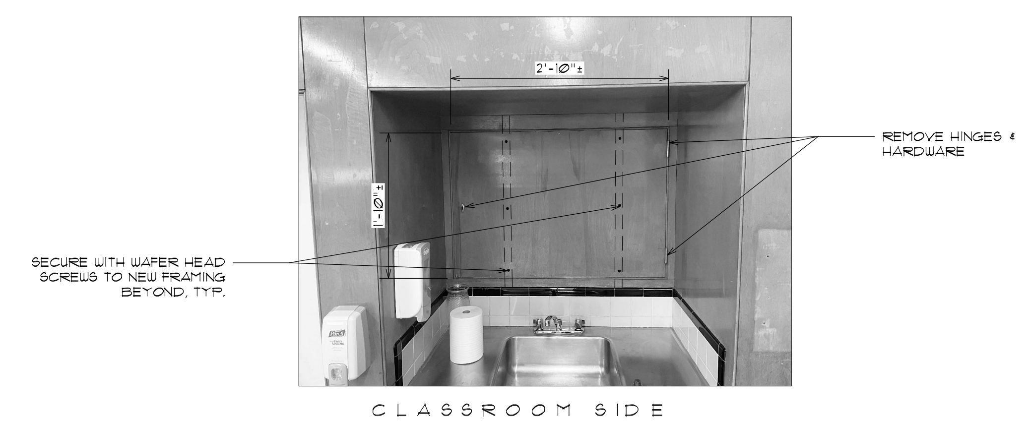
5 TYPICAL RECESSED DISPLAY CASE INFILL ELEVATION A2.2 SCALE: NTS TYPICAL AT ROOMS 109, 135, 137, 138, 140, 141, 142 & 143
