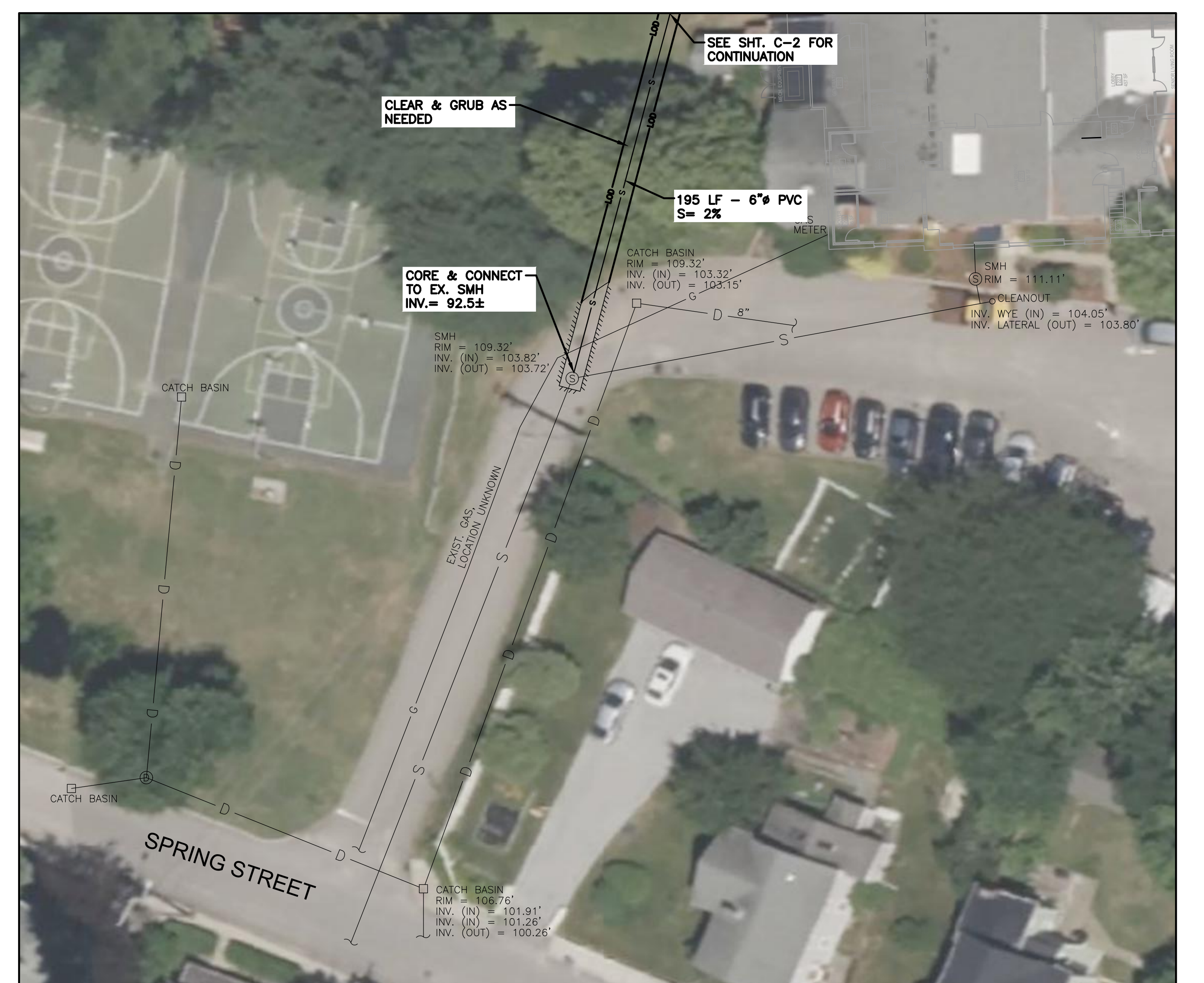
SEWER CONNECTION ALTERNATIVE NOT TO SCALE
