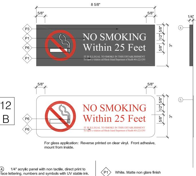
Acrylic panel shall be surface painted on front and edges. (5)Clear vinyl reverse printed decal with international no smoking symbol (red) and details of how to report a
